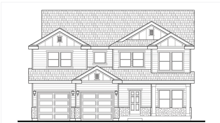
Stone, Hardie, & Stucco Exterior - Front
