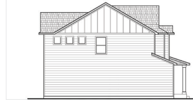
Hardie Board Exterior - Side
