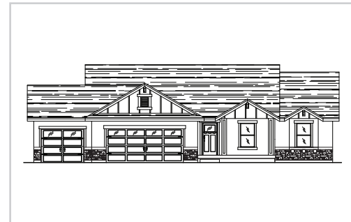
STONE AND STUCCO EXTERIOR ON ENTIRE HOME
